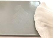
The paste electrolyte forms a purely ohmic contact between the electrode surface and the coating, therefore not interfering with the coating impedance measurement. For details of the electrolyte electrochemical characteristics and MSDS, please see the ReCorr® QCQ Paste Electrolyte documents provided with the device or contact us at <a href="mailto:info@recorrtech.com">info@recorrtech.com</a>.
